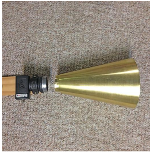
Figure 4 The configuration of the extension horn antenna as it attaches to the end of the small horn on the LNB
