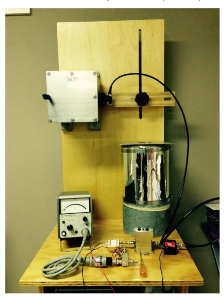
Antenna pointed into ambient temperature box with microwave absorber material inside.
