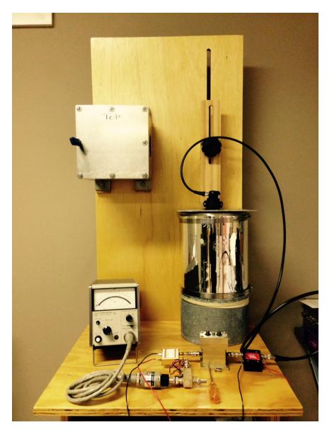
Antenna pointed at the Dewar Flask filled with liquid nitrogen. Microwave absorber material in the bottom
