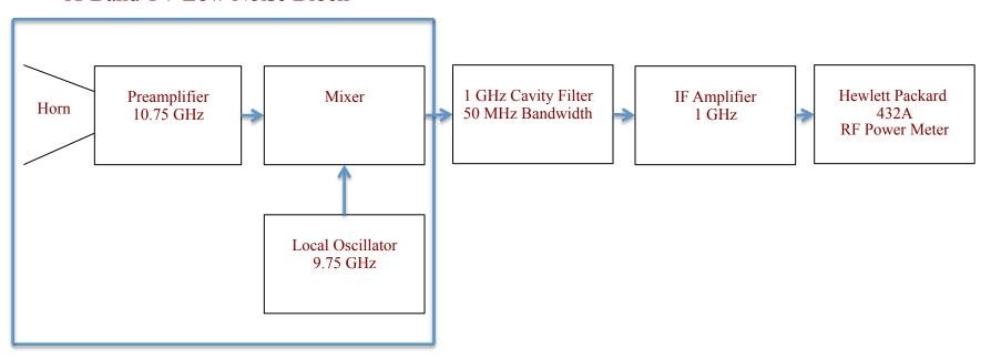
This receiver is built with parts purchased on ebay. It is a heterodyne receiver with tuned to 10.75 GHz by the choice of the 1 GHz IF filter and amplifier. There are numerous other configurations that could be used, such as a commercial 1 GHz receiver. Also, the IF section could be replaced by a software defined receiver with a a software sound power detector.
