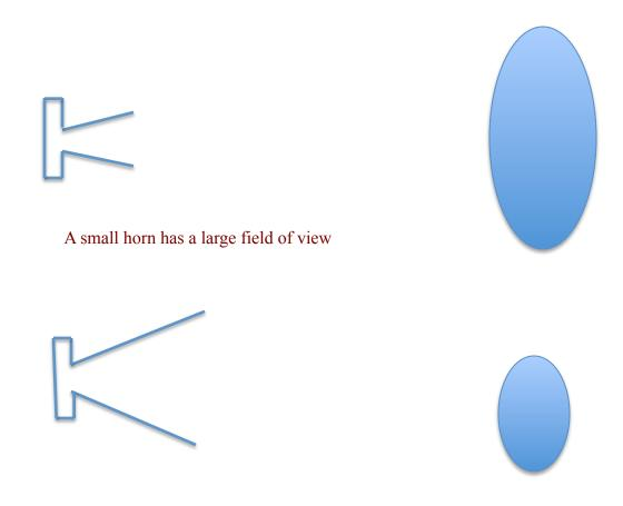
A large horn has a small field of view
