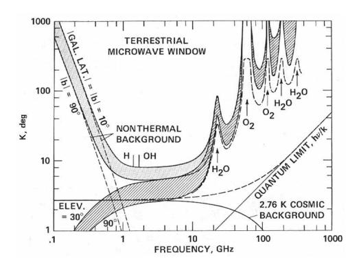
Detection is limited at low frequencies by galactic noise. Above 20 GHz, background noise from water and oxygen emission in the atmosphere limits detection. A frequency of 10 GHz has a clear window and is compatible with inexpensive electronics.
